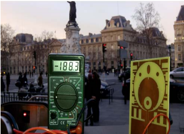
Fig. 16 – Measurement of the proposed rectenna output dc voltage as a function of the ambient RF signal harvesting in urban environments.
