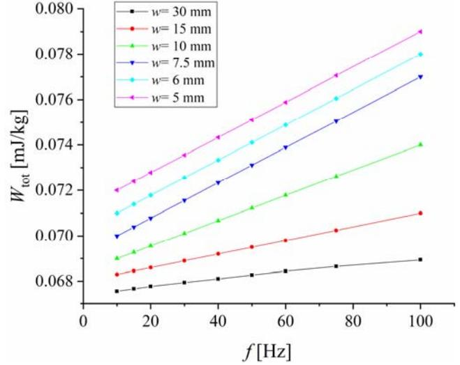
Fig. 4 – Total energy losses  $W_{tot}$  measured as a function of the frequency at  $J_p = 500$  mT for the 0.30 mm Permimphy in cold rolled state. The strip width was varied between 5 mm and 30 mm. An increase of the total energy losses, directly proportional with the frequency and inversely proportional with the strip width, can be noticed.
