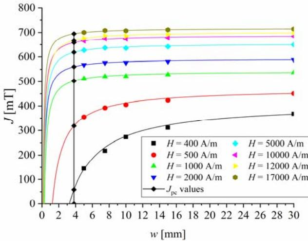
Fig. 3 – Experimentally determined magnetic polarizations  $J$  (represented with symbols) for the 0.30 mm Permimphy in cold rolled state *versus* strip width  $w$ . The solid lines are computed according to (1). The vertical line was set for  $w = 2L_c$  and the diamond symbols represent the intersection between hyperbolic dependences and the width of the entire damaged strip and correspond to parameter  $J_{pc}$ .
