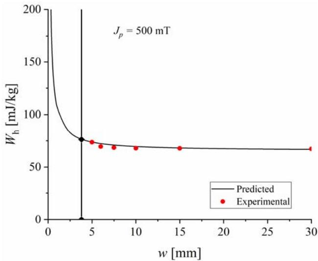
Fig. 5 – Hysteresis losses  $W_h$  as a function of the cut strip width  $w$  at  $J_p = 500$  mT for the 0.30 mm Permimphy in cold rolled state. The values computed by (3) are represented with solid lines and the experimentally computed losses are marked using the circle symbols. The black vertical line was set for  $w = 2L_c$  and the diamond symbol represent the intersection between the hyperbolic dependency and the width of the entire damaged strip ( $W_{hc}$  parameter).
