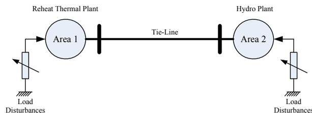
Fig. 1 – Schematic diagram of the two-area interconnected hydro-thermal system.
