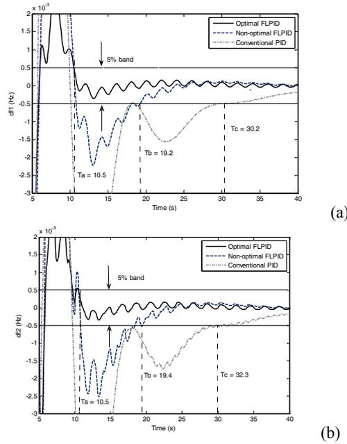
Fig. 9 – The frequency deviation of both areas in a larger scale and settling time for optimal FLPID ( $T_a$ ), Non-optimal FLPID ( $T_b$ ), and conventional PID ( $T_c$ ); a) reheat thermal area; b) hydro area.
