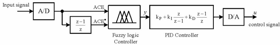
Fig. 3 – Structure of FLPID controllers in discrete mode.
