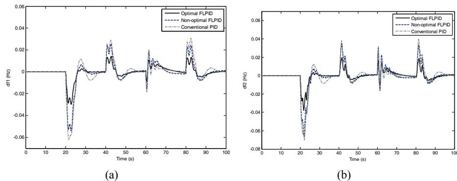
Fig. 12 – Time response of  $\Delta f_1$  and  $\Delta f_2$  under random load change:
