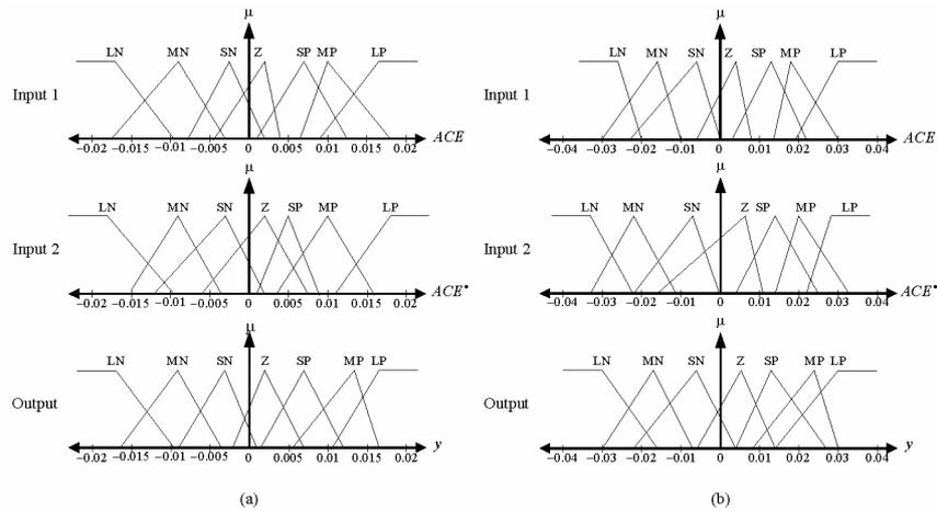
Fig. 6 – Optimized MF for optimal FLPID controllers:
