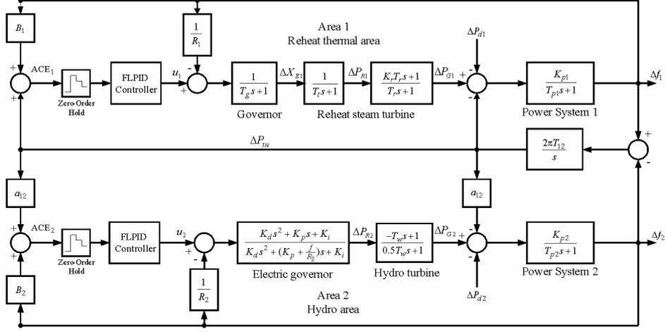
Fig. 2 – Two-area interconnected hydro-thermal system with digital controllers.
