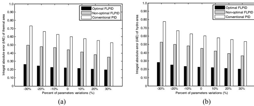
Fig. 10 – Comparison results of IAE of both areas under parameters variations: a) reheat thermal area; b) hydro area.
