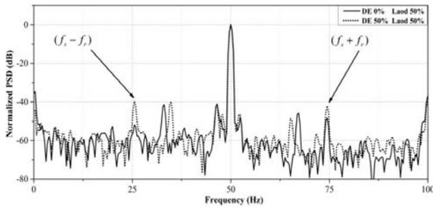
Fig. 6 – Normalized power spectrum density of stator current for case B.
