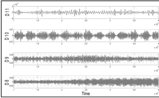
Fig. 9 – Details and approximations for eccentric machine case A.
