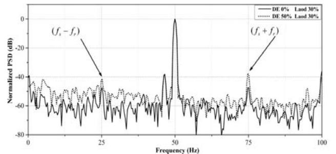
Fig. 5 – Normalized power spectrum density of stator current for case A.
