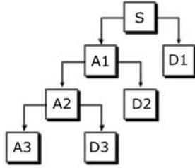
Fig. 2 – Tree decomposition of the signal S using DWT.
