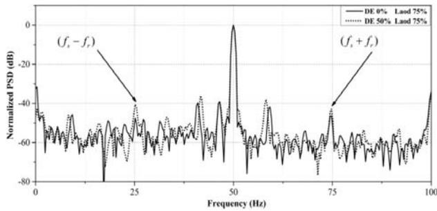
Fig. 7 – Normalized power spectrum density of stator current for case C.
