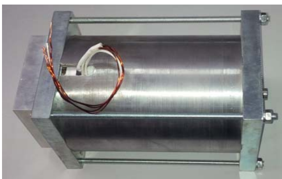
Fig. 7 – The prototype of the proposed linear dc actuator.
