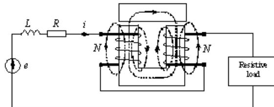
Fig. 6 – Series filter reactor.
