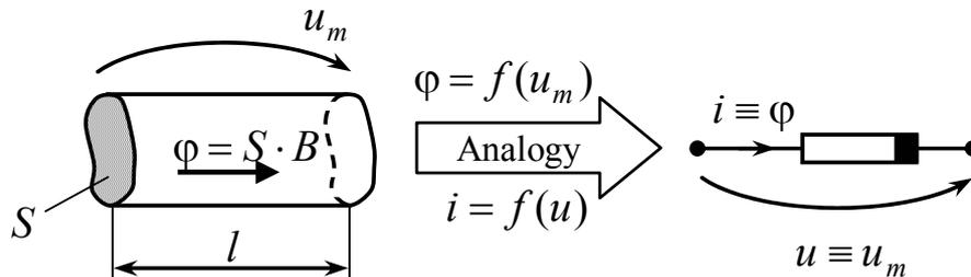
Fig. 1 – Modeling of a ferromagnetic piece, with ignoring eddy currents.
