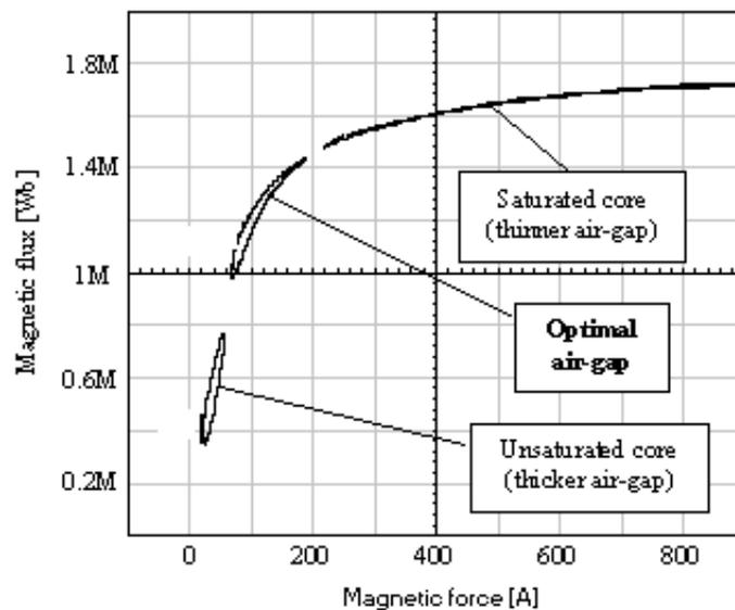
Fig. 8 – Magnetization cycles of the inductor core for three different values of the air-gap.
