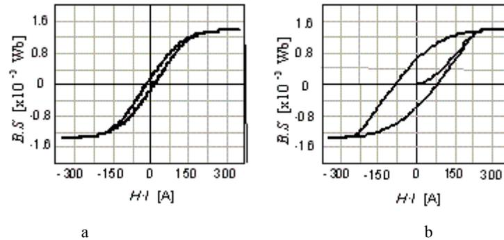
Fig. 5 – Example of a lossy nonlinear characteristic modeled to: a) 50 Hz; b) 400 Hz.
