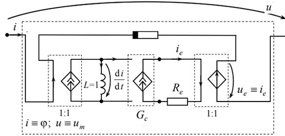
Fig. 4 – Modeling of a ferromagnetic piece, considering eddy current losses and their parasitic magnetic field.
