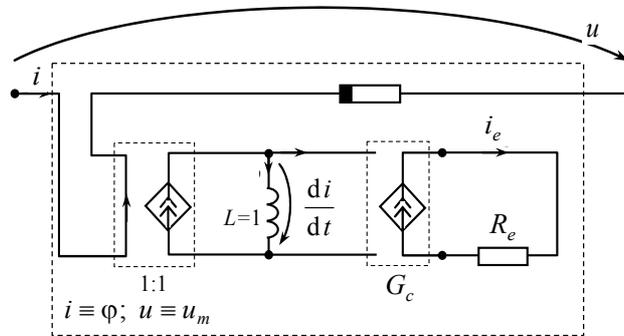
Fig. 3 – Modeling of a ferromagnetic piece, considering eddy current losses.
