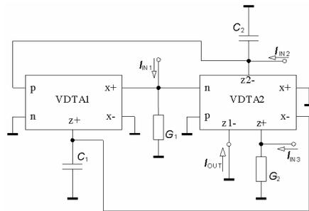
Fig. 5 – Structure of TISO universal controllable filter with two VDTAs.
