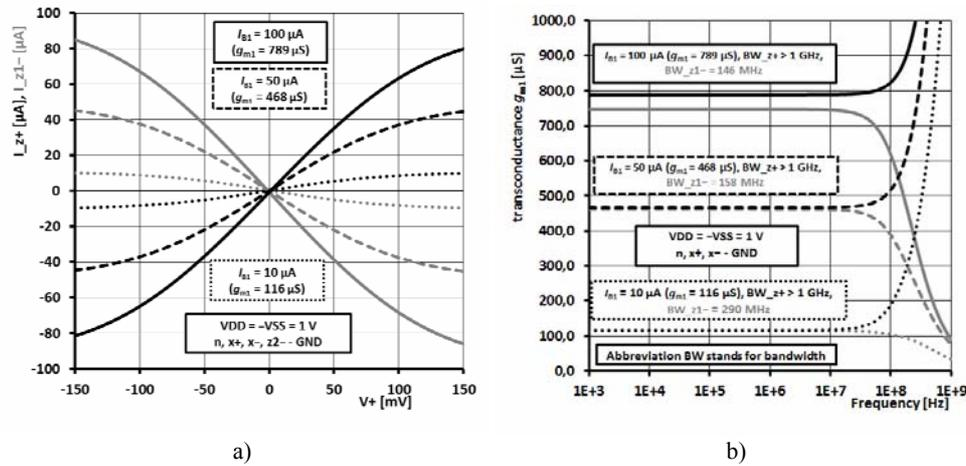
Fig. 3 – OTA performance (first section of VDTA) for selected values of control current: a) DC; b) AC. Black lines represent response on the  $z+$  output, grey lines are responses on  $z-$  output. There are three different currents (and therefore also three different  $g_{m1}$ ), first is given by solid line, second by dashed line and third by dotted line.
