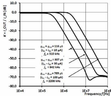
Fig. 8 – Pole frequency control with constant quality factor: Magnitude response of LP function for three different values of  $g_{m1} = g_{m2}$ .
