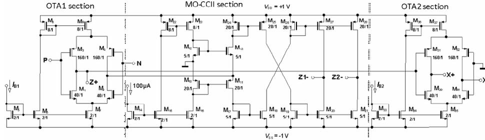
Fig. 2 – Designed CMOS implementation of proposed VDTA active element with transistor dimensions.
