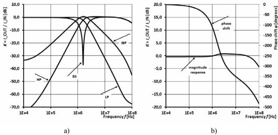
Fig. 6 – Magnitude (and phase) responses for starting parameters,  $f_p = 1.6$  MHz and  $Q = 0.707$ : a) LP, iBP, HP and BS functions; b) AP function
