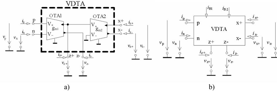
Fig. 1 – Voltage differencing transconductance amplifier (VDTA) with two independent electronically adjustable transconductances: a) basic structure; b) schematic symbol.
