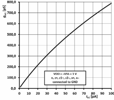
Fig. 4 – Dependence of  $g_{m1}$  of OTA (first section of VDTA) on control current.
