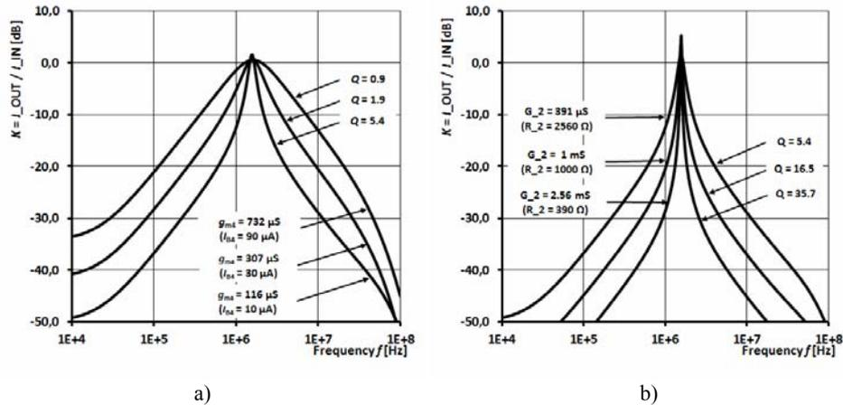
Fig. 7 – Quality factor electronic control ( $f_p = 1.6$  MHz): magnitude response of iBP: a) for three different values of  $g_{m4}$ ; b) additional possibility of control by value of  $G_2$  (when  $g_{m4} = 10 \mu\text{A}$ ).
