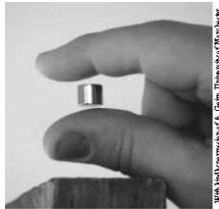
Fig. 15 – Levitation of a magnet 2.5 m below an unseen 11 T superconducting solenoid stabilized by the diamagnetism of fingers ( \chi \approx -10^{-5} ).
