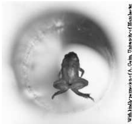
Fig. 14 – A living frog flying inside a Ø32 mm vertical bore of a Bitter solenoid in a magnetic field of about 16 T at the Nijmegen High Field Magnet Laboratory.
