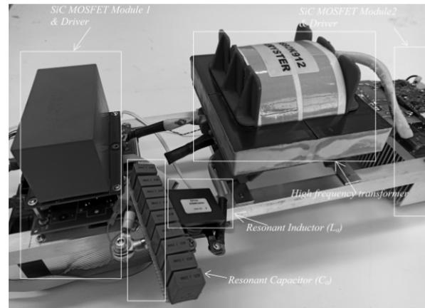
Fig. 16 – Photograph of SiC MOSFET DAB converter laboratory setup.
