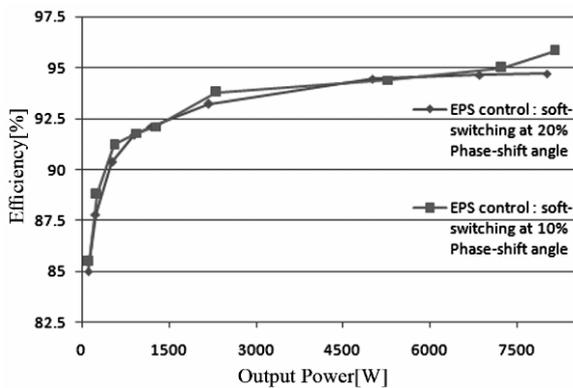
Fig. 14 –Efficiency comparisons of EPS control : soft-switching.
