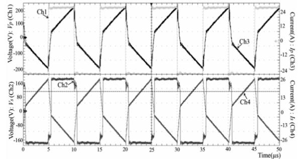
Fig. 8 –Voltage waveforms of primary and secondary side of the transformer (Ch1 : 100 V/div , Ch2: 80 V/div) and Current across the transformer primary ( $I_p$ ) and secondary ( $I_s$ ) (Ch3: 12 A/div Ch4 : 13 A/div) : DAB operated under hard switched : SPS control.
