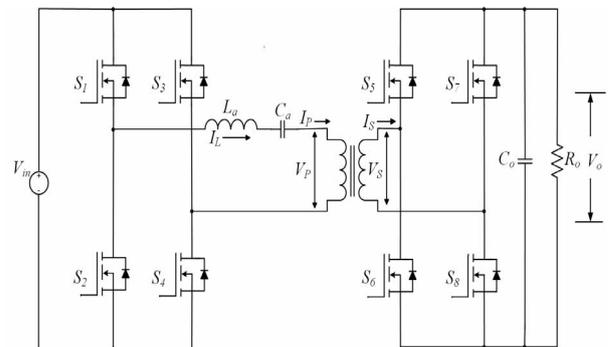
Fig. 2 – SiC MOSFET dual active bridge (DAB) dc-dc converter with series resonant network.
