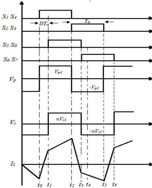
Fig. 3 – Single phase shift control key waveforms.
