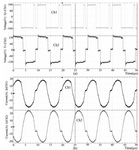
Fig. 12 – (a) Voltage waveforms of primary and secondary side of the transformer (Ch1 : 80 V/div , Ch2: 60 V/div) (b) Current across the transformer primary ( $I_p$ ) and secondary ( $I_s$ ) (Ch1: 10 A/div Ch2 : 10 A/div) : DAB Soft-switched : DPS control.
