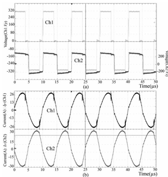
Fig. 10 – (a) Voltage waveforms of primary and secondary side of the transformer (Ch1 : 80 V/div , Ch2: 200 V/div) (b) Current across the transformer primary ( $I_p$ ) and secondary ( $I_s$ ) (Ch1: 13 A/div Ch2 : 15 A/div) : DAB with series resonant : EPS control.
