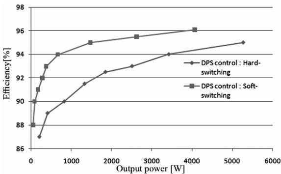
Fig. 15 –Efficiency comparisons DPS control : hard-switching *versus* soft-switching.
