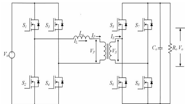
Fig. 1 – SiC MOSFET based dual active bridge (DAB) dc-dc converter.
