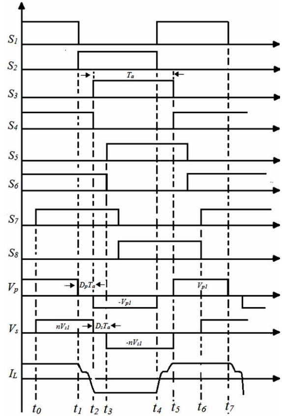
Fig. 5 – Dual phase shift control key waveforms.
