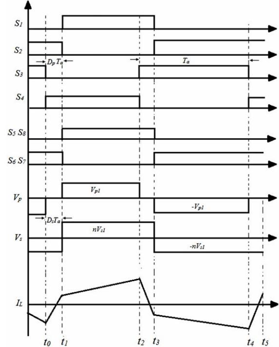
Fig. 4 – Extended phase shift control key waveforms.
