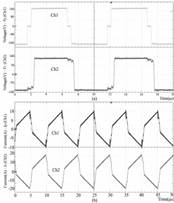
Fig. 9 – (a) Voltage waveforms of primary and secondary side of the transformer (Ch1 : 80 V/div , Ch2: 70 V/div) (b) Current across the transformer primary ( $I_p$ ) and secondary ( $I_s$ ) (Ch1: 9 A/div Ch2 : 10 A/div) : DAB operated under hard switched : EPS control.
