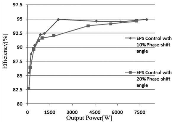
Fig. 13 –Efficiency comparisons of EPS control : hard-switching.
