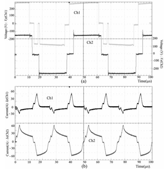
Fig. 11 – (a) Voltage waveforms of primary and secondary side of the transformer (Ch1 : 100 V/div , Ch2: 100 V/div) (b) Current across the transformer primary ( $I_p$ ) and secondary ( $I_s$ ) (Ch1: 30 A/div Ch2 : 30 A/div) : DAB hard switched : DPS control.
