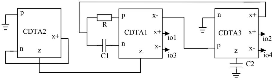
Fig. 4 – Proposed current-mode QO with the CDTA-based first-order allpass filter.
