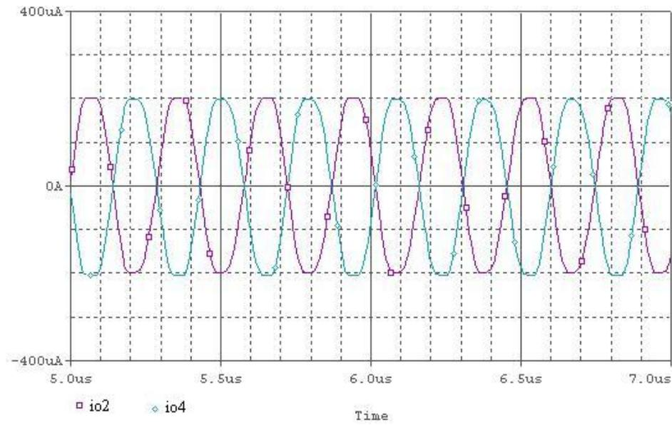
Fig. 6 – Simulated  $i_{o2}$  and  $i_{o4}$  of the oscillator.
