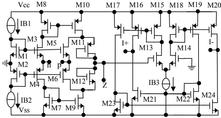
Fig. 2 – CMOS-based CDTA in this work [24].
