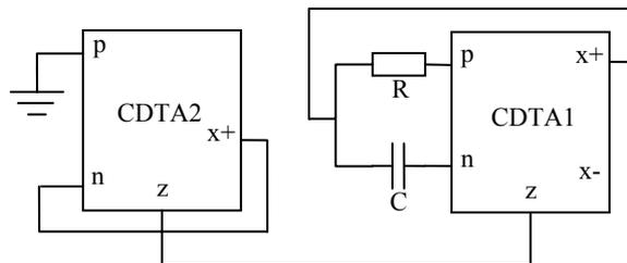
Fig. 3 – Proposed CDTA-based first-order allpass filter.
