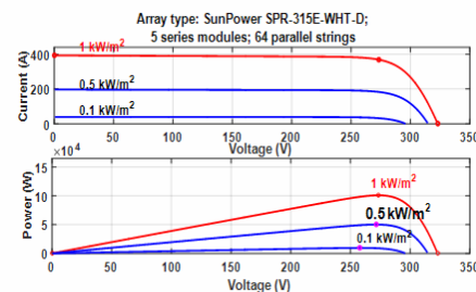
Fig. 3 – Array type: Sun Power SPR-315E-WHT-D, 5 series modules, 64 parallel strings.
