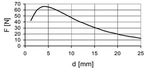
Fig. 4 – The force along  $z$  direction depending on the distance between conductive plate and permanent magnet.
