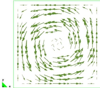
Fig. 3 – Eddy current distribution at  $t = 10$  ms.
